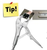
It is helpful when inserting the track into the splices to <u>lightly</u> clamp a pair of vice grips onto the track about 4" from the end of the track. This narrows the track and allows easy insertion of the splices. Don't pinch too hard or you will deform the track.
