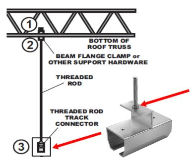
Place a nut and washer onto the rod, then place the connector and finally another washer and nut. Once the connector is level with all other connectors in the assembly, tighten the top nut to lock the hardware in place.
