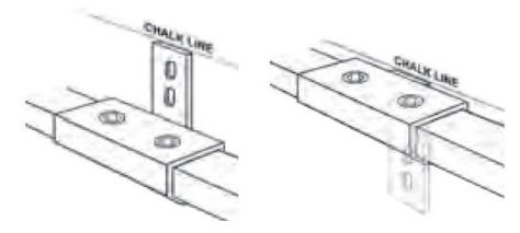
**STEP 2 -** Mark the 2 mounting holes for each of the Support Connectors.
