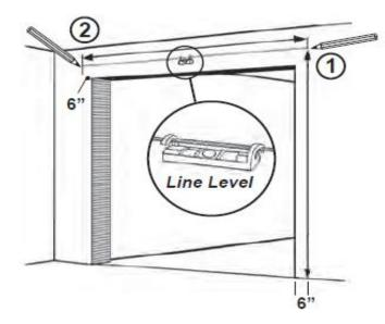
**Step 3** - Using a Line Level, place a mark on the header at least 6" beyond the opposite jamb.
