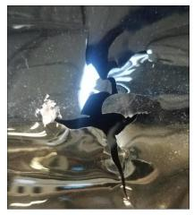
If it is cold outside then let the curtains sit for 24 hours at room temperature so that they can warm up. All PVC material can crack when it is cold as it becomes more brittle. This is very true for folded PVC which is required for shipping as there is a lot of stress *on the folds*.
