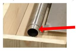
The ends of the track will fit inside each other with the sleeve design.
