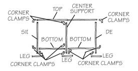
On frames wider that 8', we include an additional center support. Therefore, instead of usual 4 pieces of tubing, the wider frame will have 6 pieces. Three pieces will be of equal length. These are the 2 SIDES and CENTER SUPPORT. There will be 1 long piece for the TOP and 2 short pieces for the <u>BOTTOM</u>. In addition, there will be 3 <u>LEGS</u>. In addition there will be 10 CORNER CLAMPS
