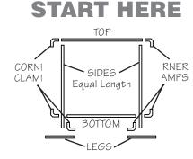
All frames up to 8' in width have 6 pieces of <u>SQUARE TUBING</u> and 6 <u>CORNER</u> <u>CLAMPS</u>. The two pieces of tubing that are of equal length, are the <u>SIDES</u>. Of the remaining pieces, the longer piece is the <u>TOP</u>; the shorter piece is the <u>BOTTOM</u> and fits inside the two side pieces. The last two pieces are the <u>LEGS</u>.
