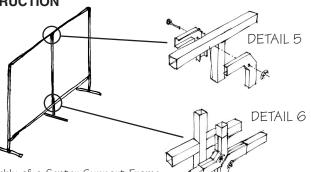
Assembly of a Center Support Frame is very similar to normal frame construction.
