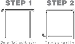
On a flat work surface, layout the 2 side pieces and top piece as shown above. Attach the corner clamps at both corners with the top
